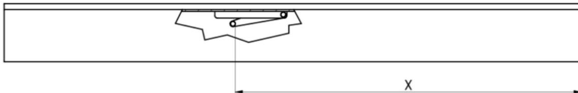
First screw the trigger to the track with 2 screws as shown, and then a single screw through the trigger to gently secure. This last single screw and the grub screw allows you to adjust the height of the bar if required.
