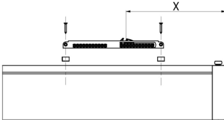
Mount the trigger in the top track at the same distance from the end of the track you have just measured.
