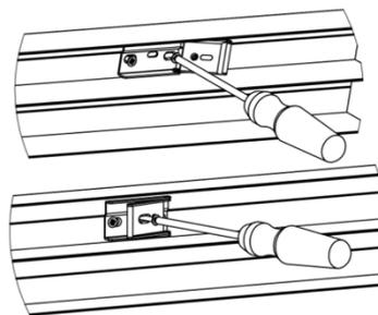
Adjust the height of the door, so the soft close damper meets the trigger.
