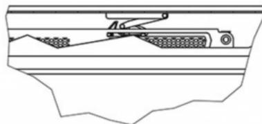
Adjust the height of the door, so the soft close damper meets the trigger.
