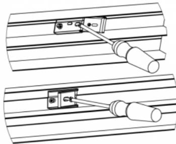
This last single screw and the grub screw allows you to adjust the height of the bar if required.
