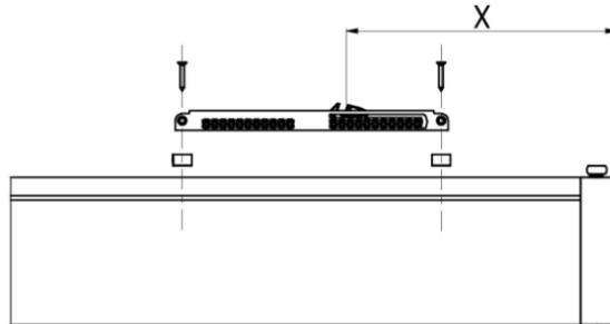
Mount the soft close trigger in the top track at the same distance from the end of the track you have just measured.
