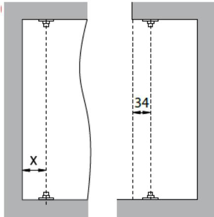
Note: When fixing the pivot base, use screws with a head diameter of not more than 8 mm.
